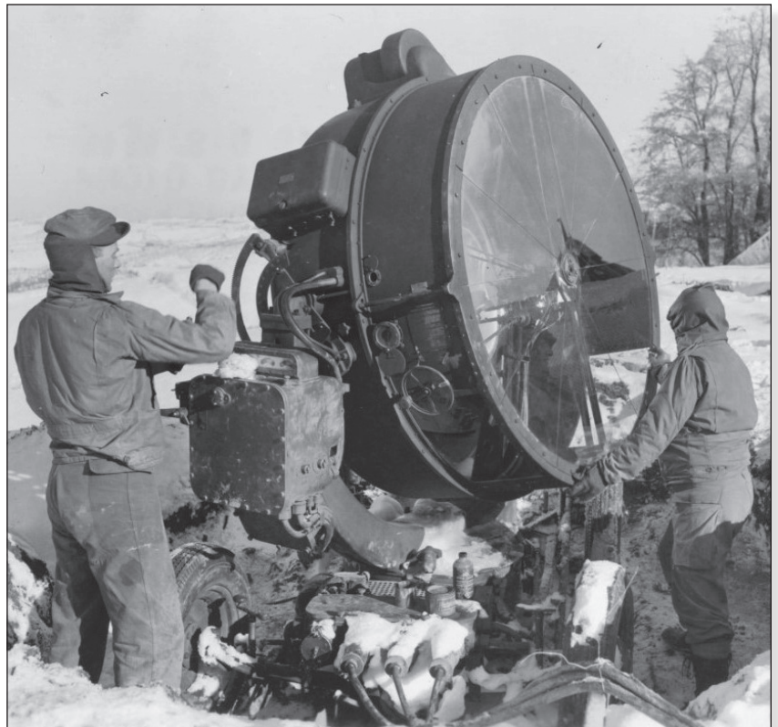
Typical army anti-aircraft searchlight from World War II, 4 or 5 feet in diameter.
